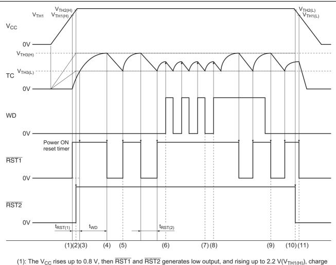
Timing Chart 1 (When the delay capacitor is not connected with Ct1 pin)
